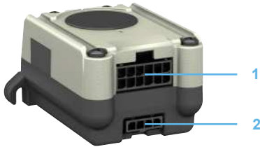
SD215DU20C drive with pulse/direction interface
