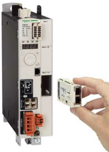
Installing the CANopen communication card VW3A3608
