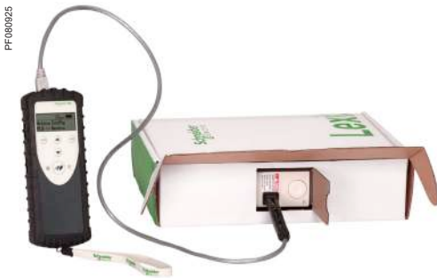
Configuration of a Lexium 32 in its packaging with the VW3A8121 Multi-Loader tool + VW3A8126 cordset
